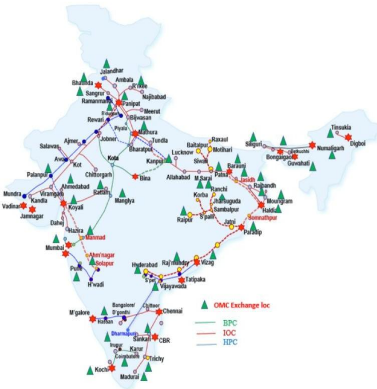
Figure 178: Map depicting POL Pipeline, Depot/Terminal & Refineries
