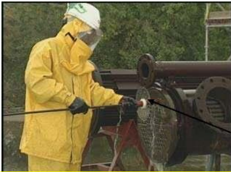
Typical anti-withdrawal device for stiff lancing
