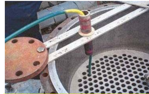
Typical anti-withdrawal device for flex lancing
