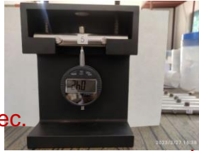
Deflection measurement with LVDT
