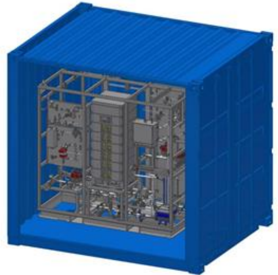
Isometric view of the artist's impression of the compression and purification system of 40 kg H 2 /day
