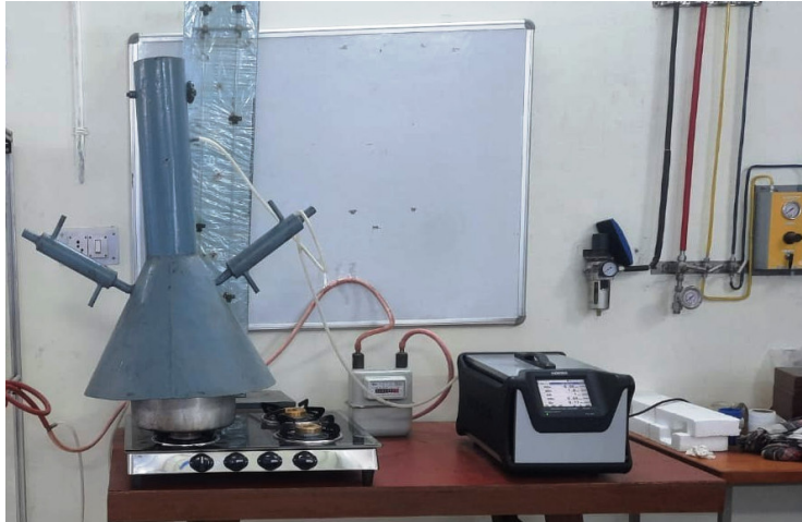
Combustion Efficiency Test Setup
