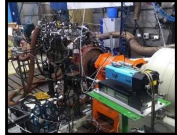
Demonstrative up-gradation of existing BS-IV NG HCV Engine to meet BS-VI emissions
