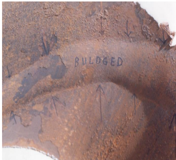
Hydrogen Fissures / Blistering in Line pipe due to H 2 / wet H 2 S Corrosion
