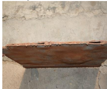
Hydrogen Fissures / Blistering in Line pipe due to H 2 / wet H 2 S Corrosion
