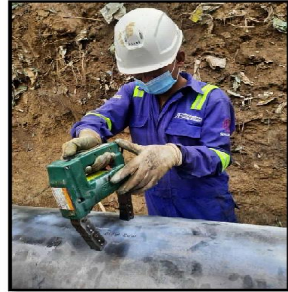
Figure 22: Magnetic Particle Inspection (MPI) for Stress Corrosion Cracking (SCC) for Pipe Body, ERW Seam as well as Girth Welds
