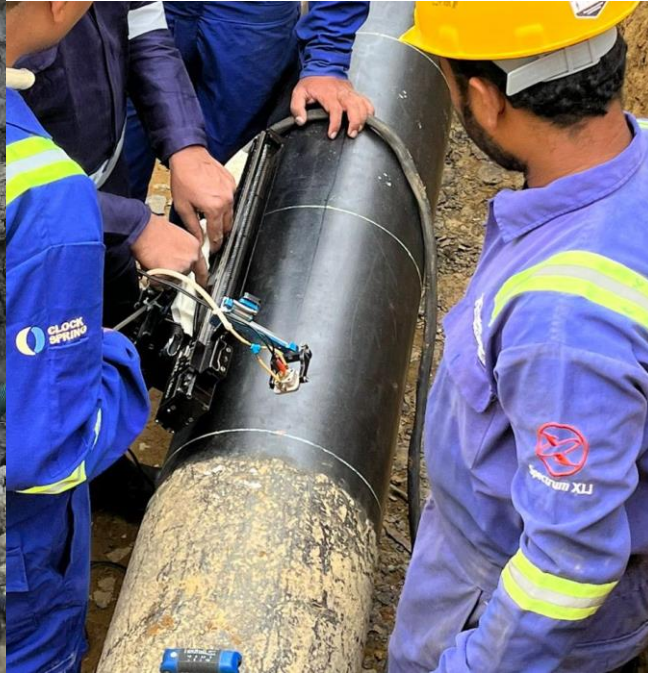
Figure 22: Magnetic Particle Inspection (MPI) for Stress Corrosion Cracking (SCC) for Pipe Body, ERW Seam as well as Girth Welds
