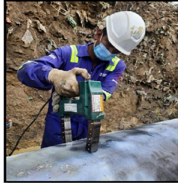
Figure 22: Magnetic Particle Inspection (MPI) for Stress Corrosion Cracking (SCC) for Pipe Body, ERW Seam as well as Girth Welds
