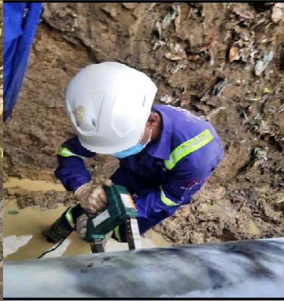
Figure 22: Magnetic Particle Inspection (MPI) for Stress Corrosion Cracking (SCC) for Pipe Body, ERW Seam as well as Girth Welds
